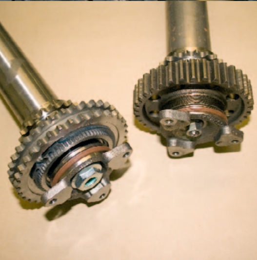
The right-hand intermediate shaft is a late-type with the large toothed sprocket. The other is Autofarm's own design which combines the later bearing with a sprocket that is compatible with the earlier twin-chain drive
