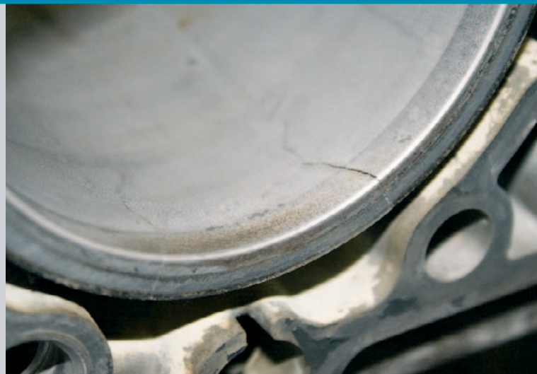
This shows a classic cylinder bore failure. Note the two parallel cracks running down the bore. In time, these can join and a 'D' shaped chunk of liner may break away
